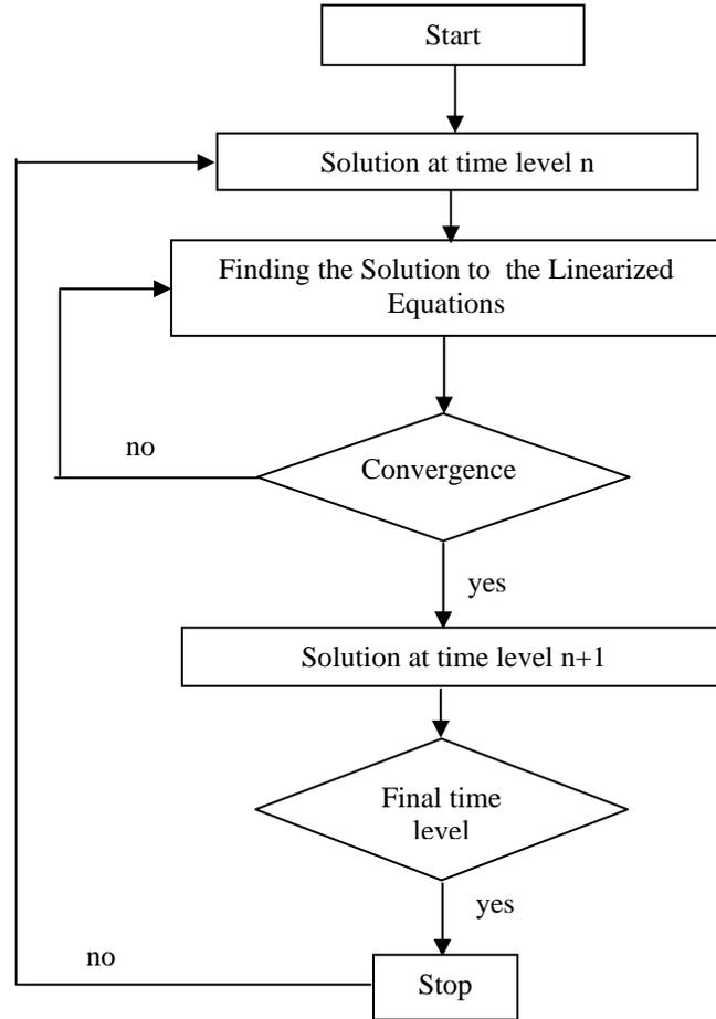
Figure 9. Solution procedure for a nonlinear set of equations.
