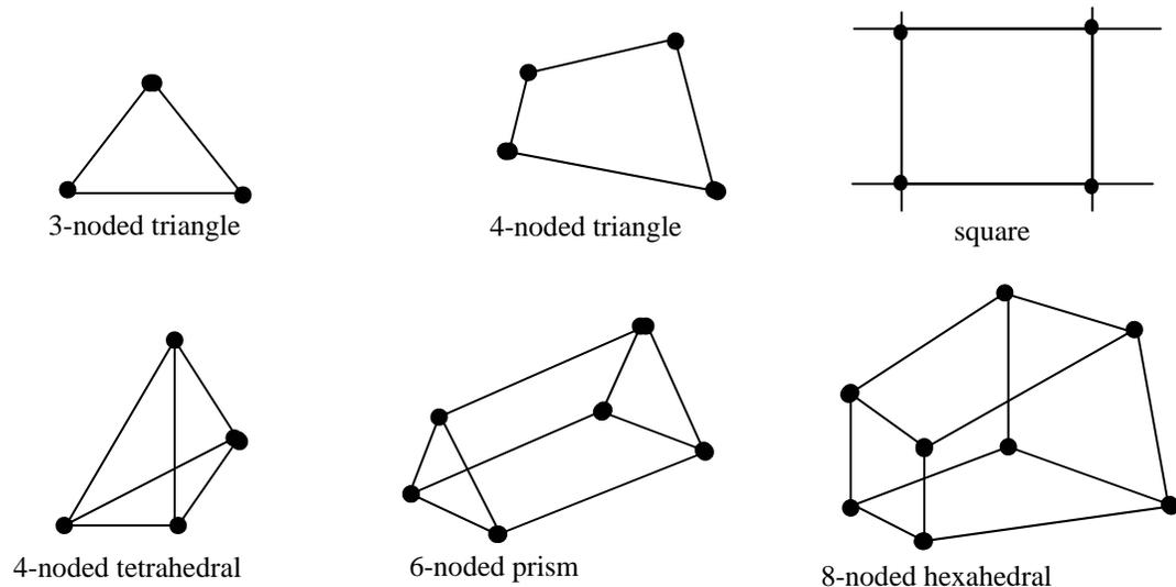
Figure 12. Typical computational elements.
