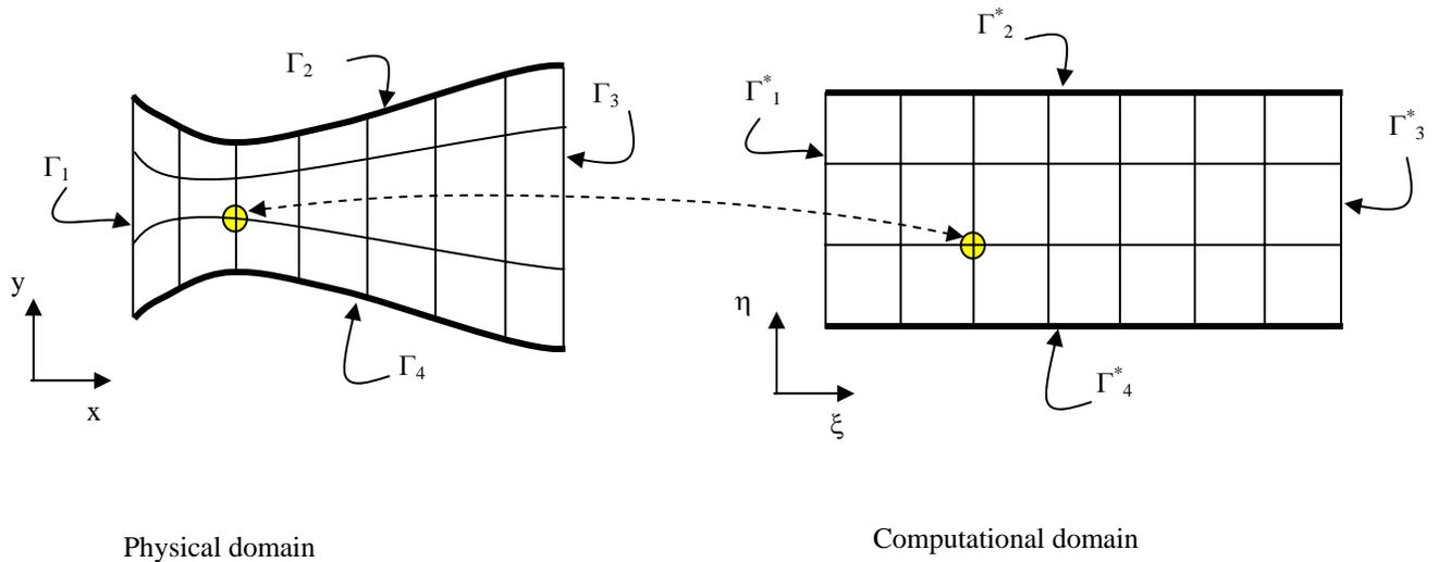
Figure 14- The Transformed Computational Domain
