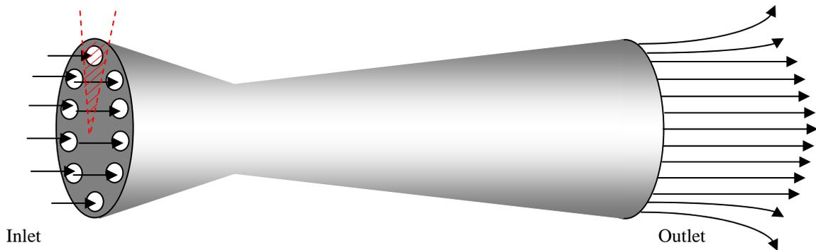
Figure 1. Schematic of the flow inside and outside of a converging-diverging nozzle
