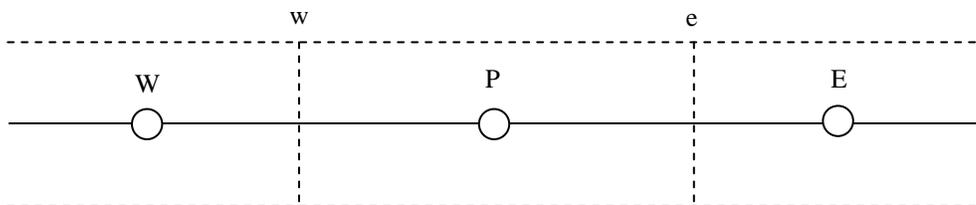
Figure 6. A finite volume in one dimension.
