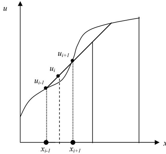
Figure 5. A two-noded linear element
