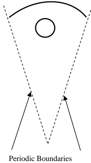
Figure 2. Minimizing the computational domain using periodic boundary condition
