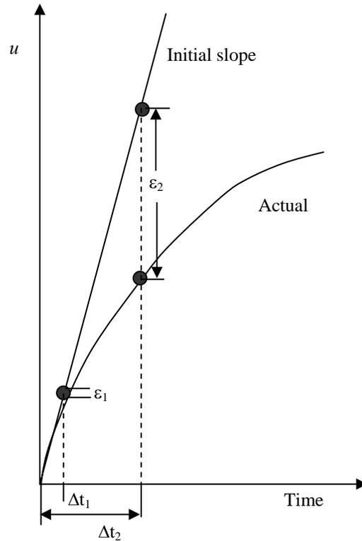
Figure 10. The influence of the time step on the solution.
