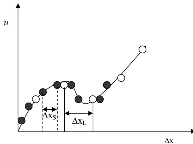
Figure 13. Coarse and fine mesh representation of function  $u$ .
